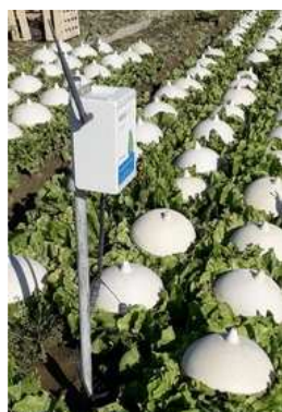
Sonde capacitive, photo CA31
